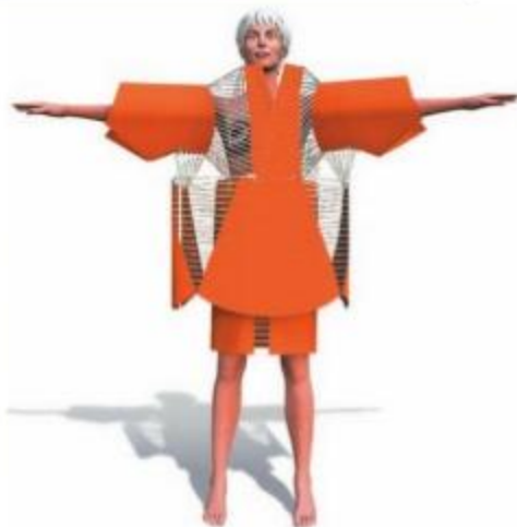
The 3D program Vilna . The positions are shown where the garment pieces have to be 'virtually stitched' together. Illustration by permission of assyst-bullmer.
