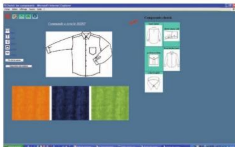
Measurements taken by body scanning, and fabric and style selection for made-to-measure garments in the FitNet program. Illustrations by permission of Lectra.
