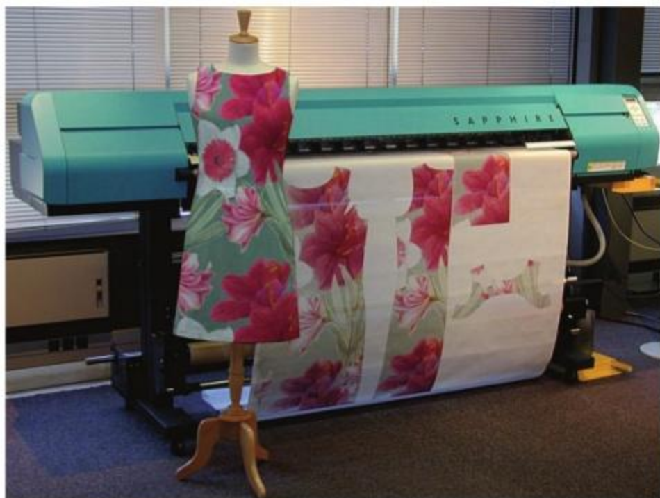
Pattern development incorporating printed textiles. Fabric pieces printed out on an inkjet printer and then made up into sample garments. Photograph by permission of Lectra.
